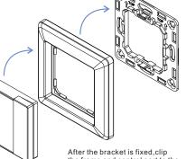
the frame and control part to the bracket in sequence
